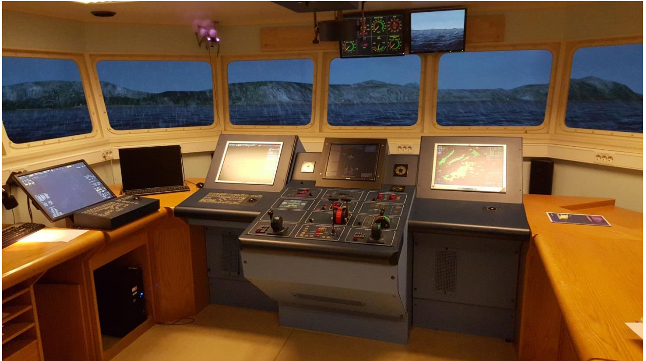
Figure 2: “Horten” Navigation Simulator at USN - Kongsberg Bridge Line 10 simulator (upgraded to K-Bridge software) with a 225° forward view (copyright author).
